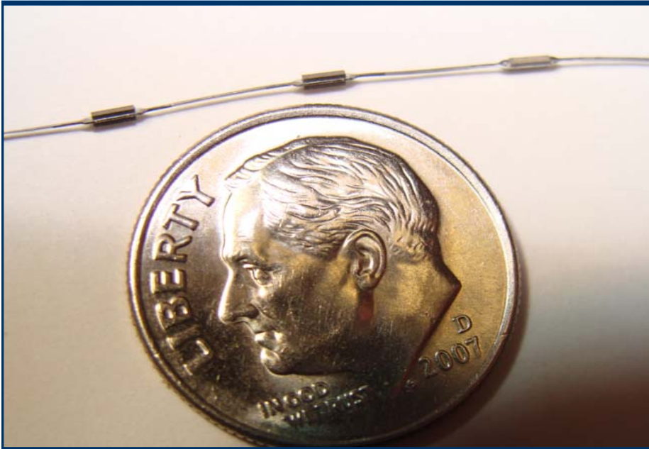
Specific design ...performance driven micro transducer (Actual size comparison with dime)
